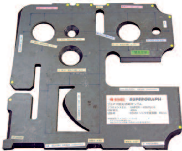
Cutting example – Versagraph with 3D-LINK
